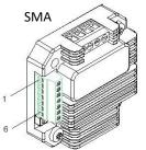
H/L must be connected to 0v for 40 & 150 rpm speed ranges. ENA, On/Off & Direction connections are optional. Pump will run clockwise once supply is connected remove to stop or alternatively connect 0v to ENA this will stop motor. Connecting 0v to ON/OFF will also stop the motor but it is a powered stop/hold so motor will remain powered all the time causing additional heat generation.
