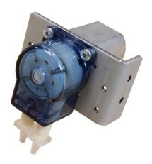
The 100 series, micro range of peristaltic pumps offer a low cost, compact & reliable means of dosing a wide range of liquids. They are available in various configurations of tubing type & size giving flow rates of between 0.016 & 0.26 ml/rev. The pump head is designed to be disposable but is assembled using a single screw enabling dis-assembly & re-assembly for tube changing if required.
