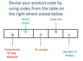
102-015-230-016/4 Example product code for 100 series pump head fitted with Viton® tubing , 15 RPM, 230v AC, 1.6mm ID tubing & 4 rollers
